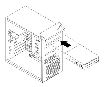
Figure 19. Installing the optical drive
